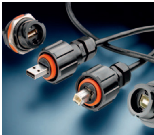
▲ Figure 3: Circular sealed USB 2.0 connectors provide protection to IP67 thanks to their ¼ turn bayonet coupling ring and seal. For more information: Europe , North America , and Asia-Pacific .
