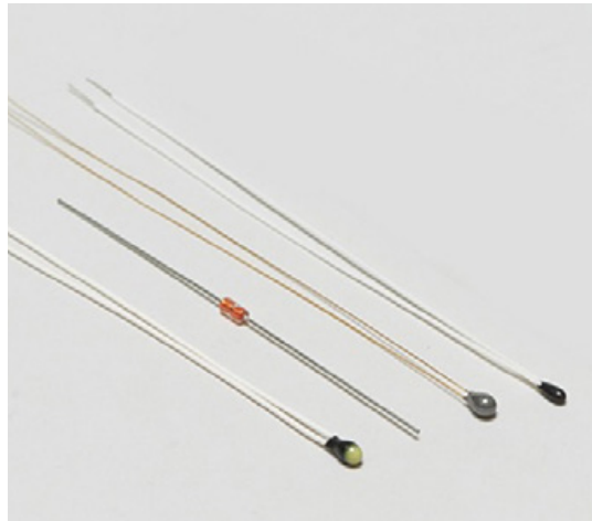
▲ Figure 3: A range of NTC thermistors suitable for -80^{\circ}\text{C} to +300^{\circ}\text{C} temperature measurement.
