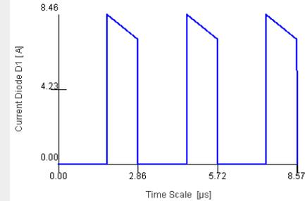
Min. Current Diode D1: 7.06 A
