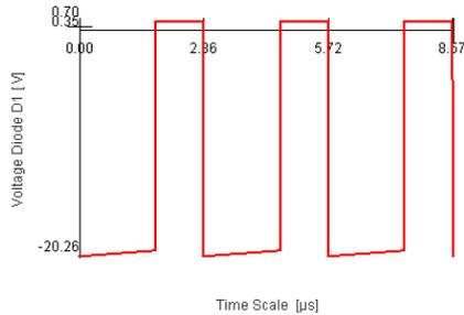
Min. Voltage Diode D1: -20.26 V
