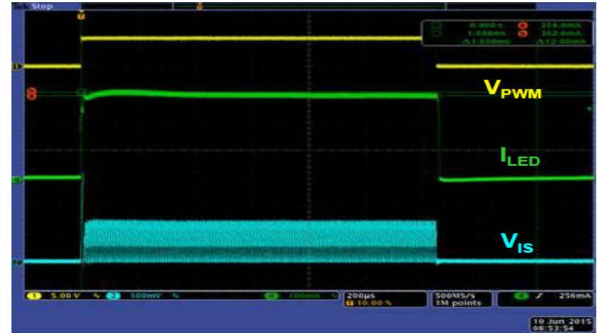
$V_{IN} = 14V$ , 18 LEDs,  $V_{IADJ} = 420mV$ ,
