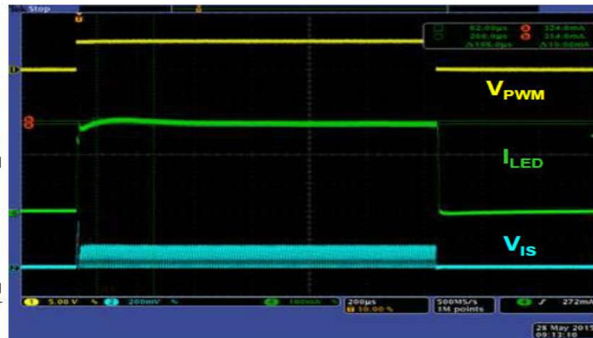
$V_{IN} = 14V$ , 18 LEDs,  $V_{IADJ} = 420mV$ ,
