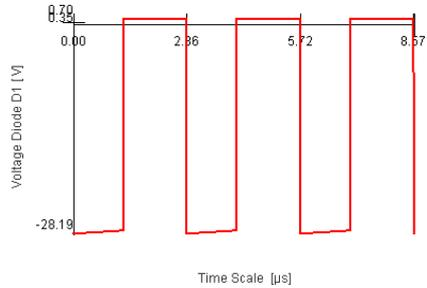
Min. Voltage Diode D1: -28.19 V
