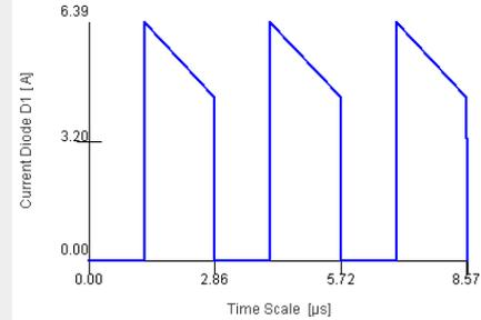
Min. Current Diode D1: 4.37 A
