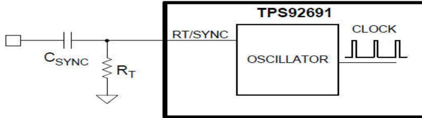
Oscillator Synchronization Through AC Coupling
