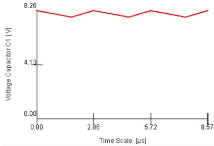
Min. Voltage Capacitor C1: 7.74 V
