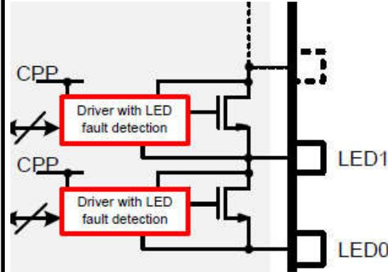
LPP's LED Matrix Manager enables convenient LED fault protection and reporting per individual LEDs
