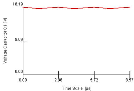
Min. Voltage Capacitor C1: 15.81 V
